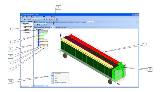
The presentation "3D View" [1] shows a step-by-step loading sequence of a vehicle in a 3D format. In the left corner of the window, the user can see a sequence of steps of the loading [2] and information about the boxes that are loaded at each particular step that includes:
