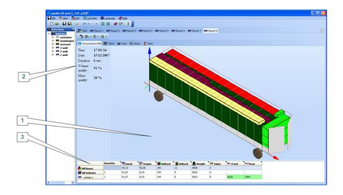
In presentation "Document profile" the central part of window is occupied by a 3D-view of a loaded vehicle [1]. The quality of loading as well as information about the date and duration of the calculations are shown in the table [2]. More detailed information about the way the vehicle is loaded can be viewed in the table [3].
