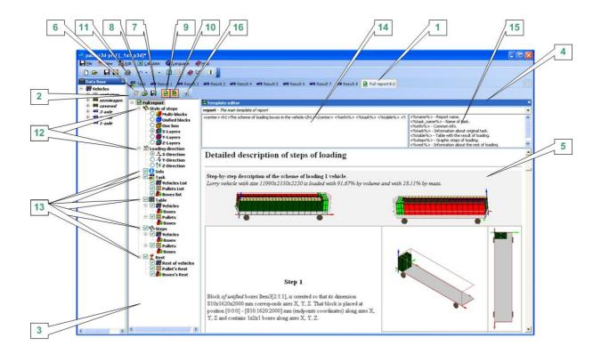
The window of the vehicle loading sequence Report [1] contains control panel [2], blueprint tree [3], blueprint editor [4], and the window with generated static step-by-step loading sequence [5] ready to be printed. Each of these elements is described in details in this section.
