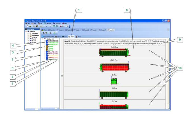
The presentation "Steps" [1] shows steps of a loading sequence of a vehicle in format of projections. In the left corner of the window, the user can select a particular step of a loading sequence [2] and see information about the boxes that are loaded at this particular step that includes:
