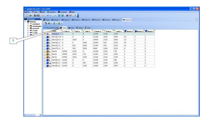
The presentation "Table" [1] contains information about step-by-step loading of a vehicle as a table. The rows of the table present steps of the loading sequence, the columns contain information about location (co-ordinates) of the boxes in the vehicle and any blocks formed of the same-type boxes.
